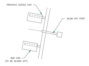
"ON" Position of Pin Chain Blow-off Solenoid
